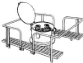
20,000 GALLON CAPACITY - INSULATED DOT 105A500W FOR CARBON DIOXIDE SERVICE (PRE 1983)
